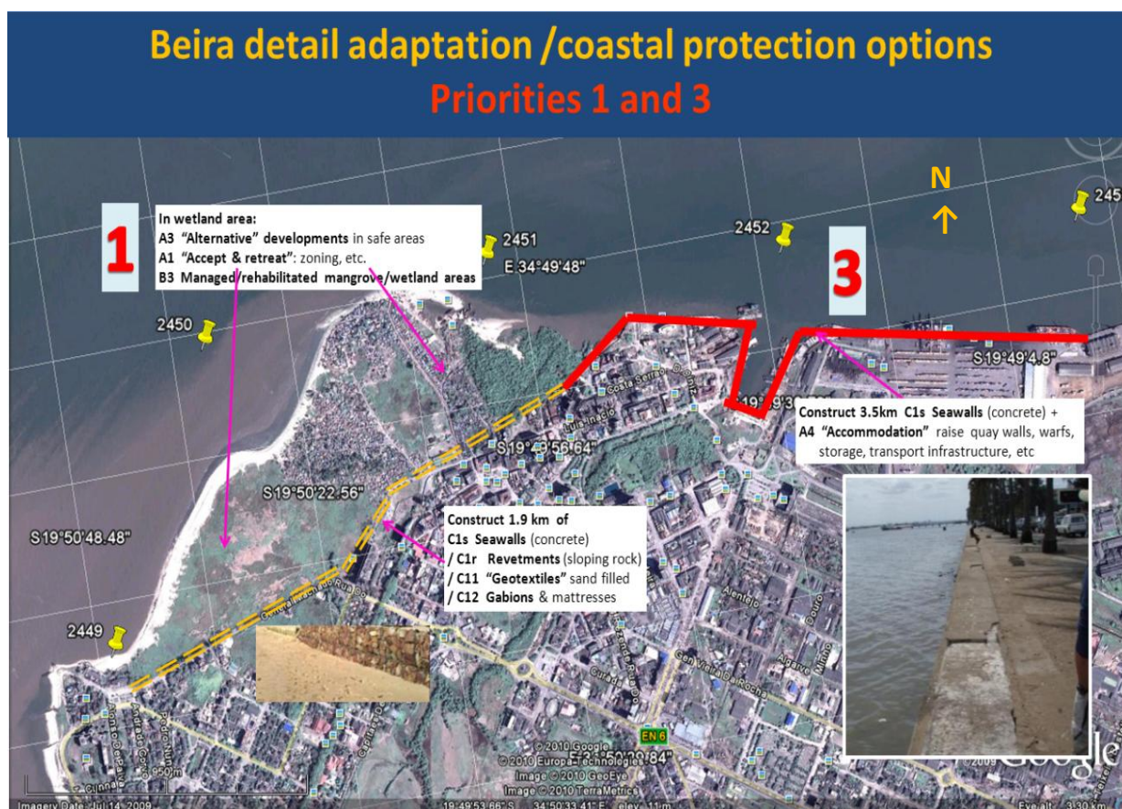
Figure 14: Western Beira: Adaptation and coastal protection options based on general criteria, local site characteristics and current use or value
