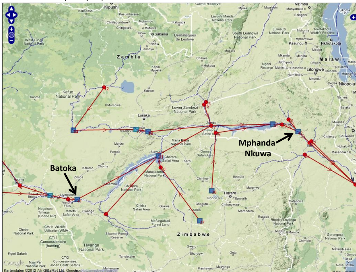
Figure 31: Computation point network for the hydropower case study, including the planned reservoirs of Batoka Gorge and Mphanda Nkuwa As can be seen from Figure 31, in the predefined hydropower scenario, the commissioning date (the year in which the operation starts) of the reservoir is set for 2020 to overlap entirely with irrigation scenario 1.
