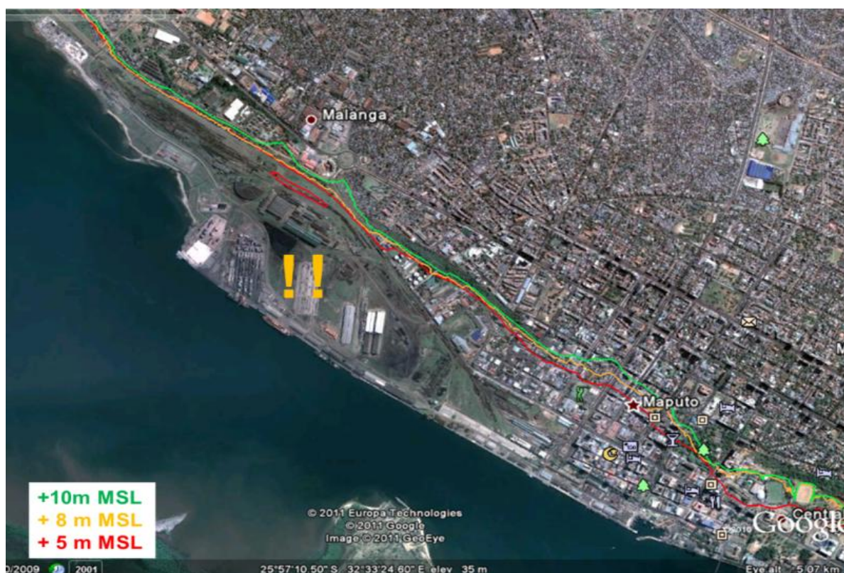
As can be seen from Figure 15B, many of the existing Maputo port and adjacent developed areas are located below the estimated +5 m MSL contour position. They are therefore already considered vulnerable to extreme events during MHWS (which occurs approximately every 14 days) and in the low climate change scenario of 0.5 m SLR by 2100, even without considering wave run-up.
